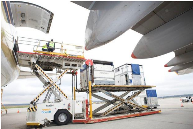
Fig. 4 Horse stalls being loaded on to a cargo plane (Photo: IRT, Magee 2015).
